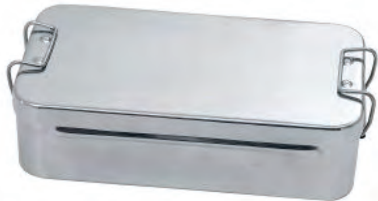
AIH-1110 Manufactured from 18/10 stainless steel Body lid and perforated internal tray pressed without welding. Hooks to lift the internal tray, closed with joint handle.
